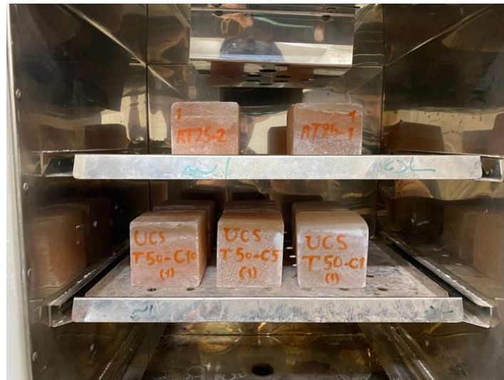
Fig. 3. Cubic rock salt specimens ready for heating to 50°C.
