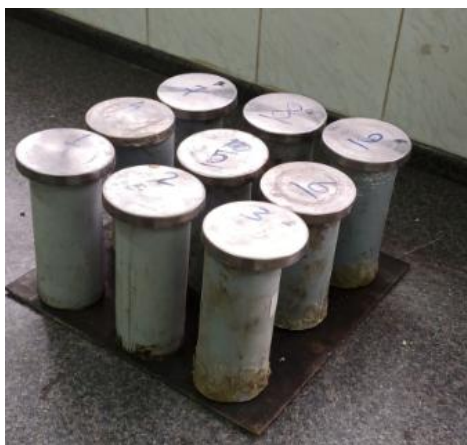
Fig. 4. The preparation method of UCS samples
