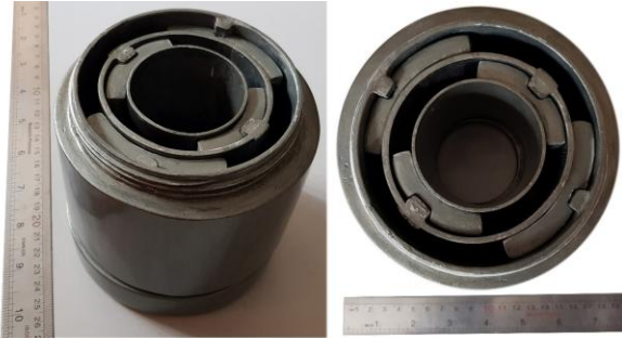
Figure 4. Prototype of cell constructed using epoxy resin
