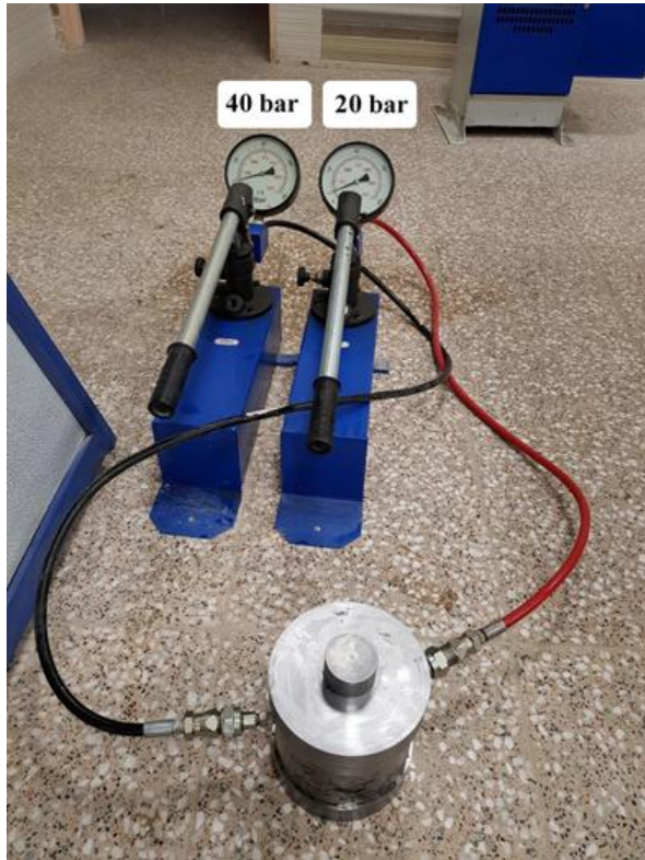
Figure 12. Connection of cell to hydraulic jacks applying different confining pressures.
