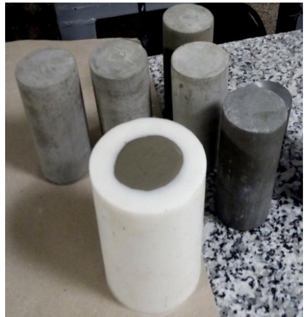
Figure 11. Concrete sample preparation
