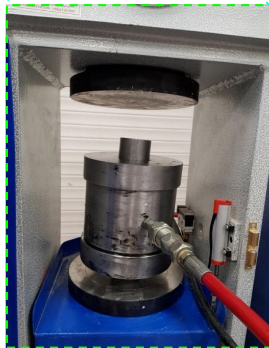
Figure 13. The setup of true triaxial test using developed cell
